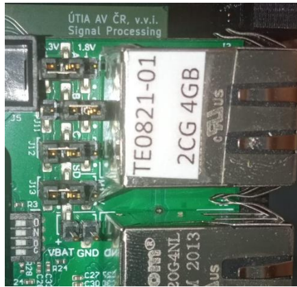
Figure 3: Jumper settings on carrier board TE0706-3
