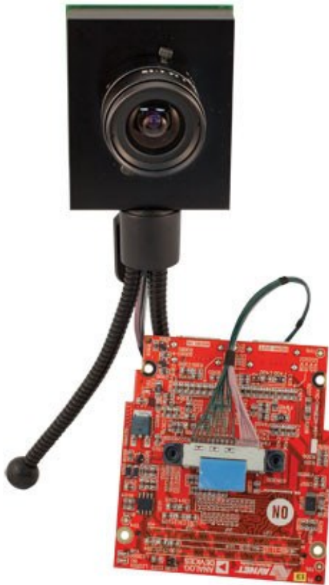
Figure 5: Avnet Vita 2000 image sensor [5].
