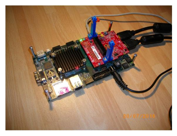
Figure 1: TE0701-05 platform, Zynq device and HDMII-HDMIO support.
