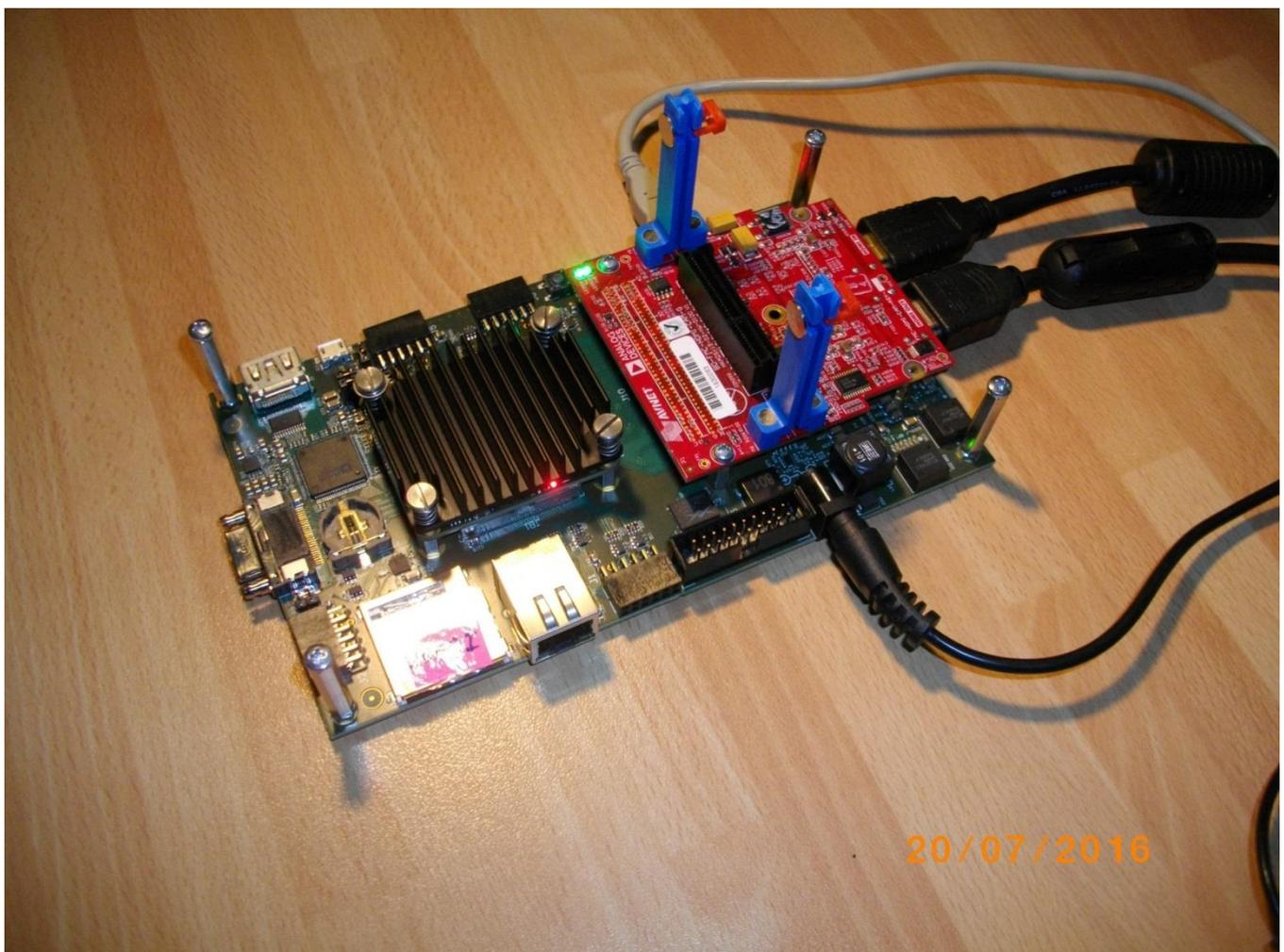
Figure 1: TE0701-05 platform with Zynq XC7Z020-2I device and HDMII-HDMI support.
