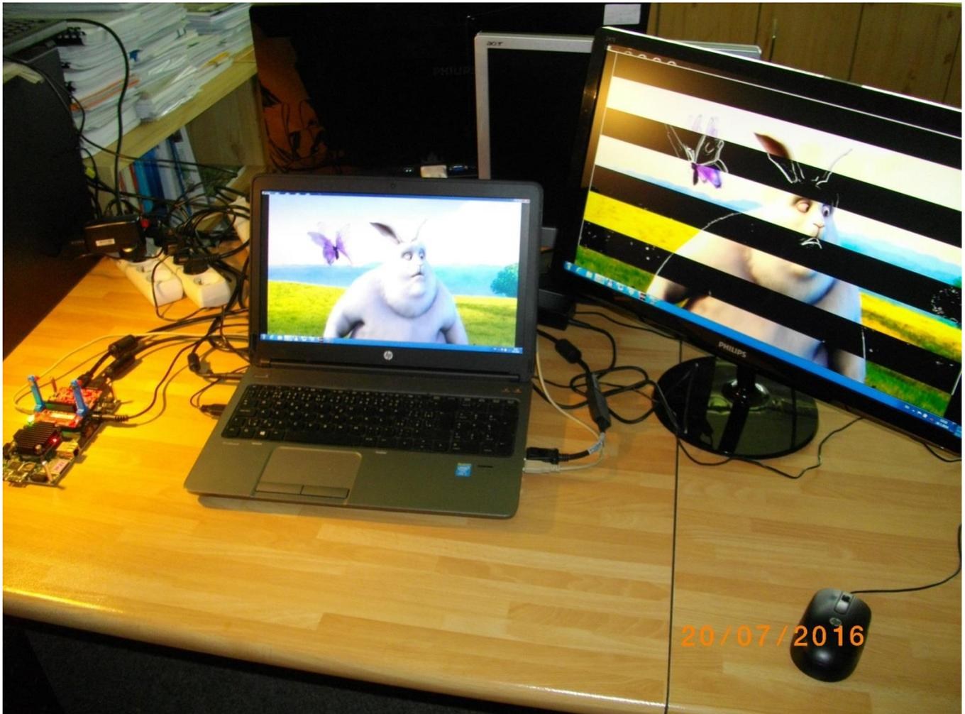
Figure 2: HW accelerated edge detection in Full HD with 4 HW paths and variable area (so04 demo).
