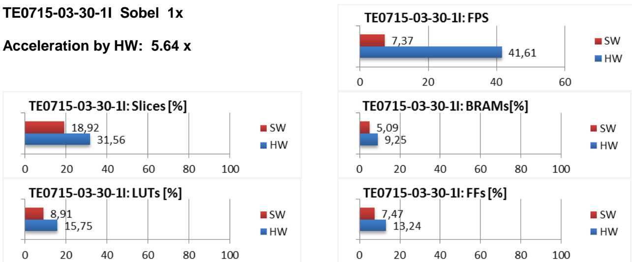
Figure 4: Project sh01 - Acceleration and HW resources used.
