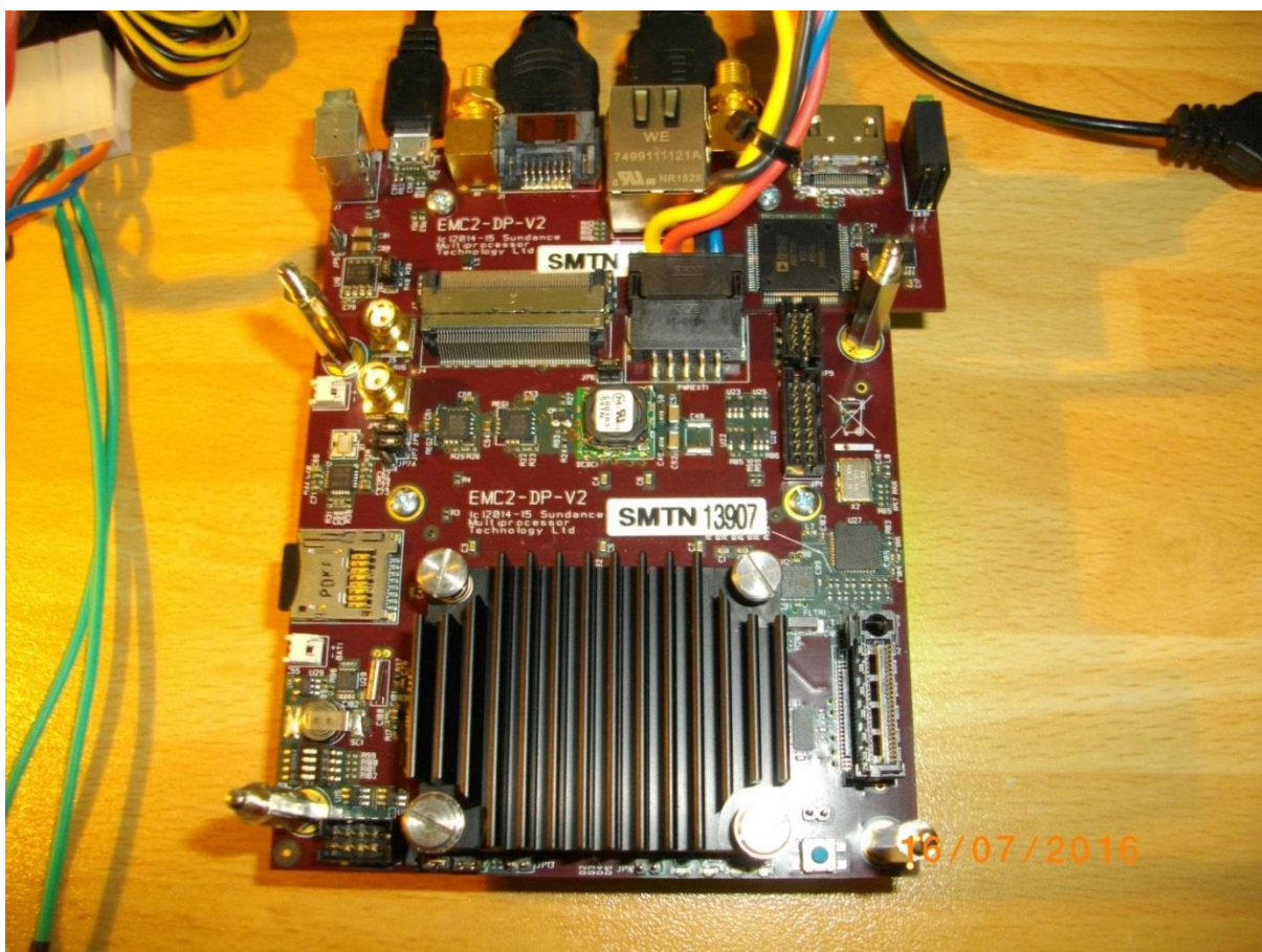
Figure 1: Sundance EMC2-DP-V2 platform with Zynq XC7Z030-1I device and HDMI-HDMI support.
