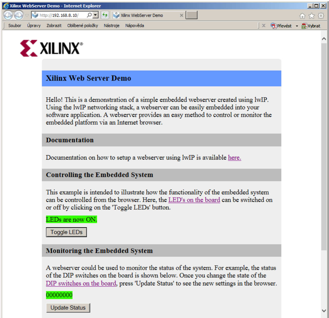
Figure 35: Start test from the web browser GUI by Toggle LEDs button.
