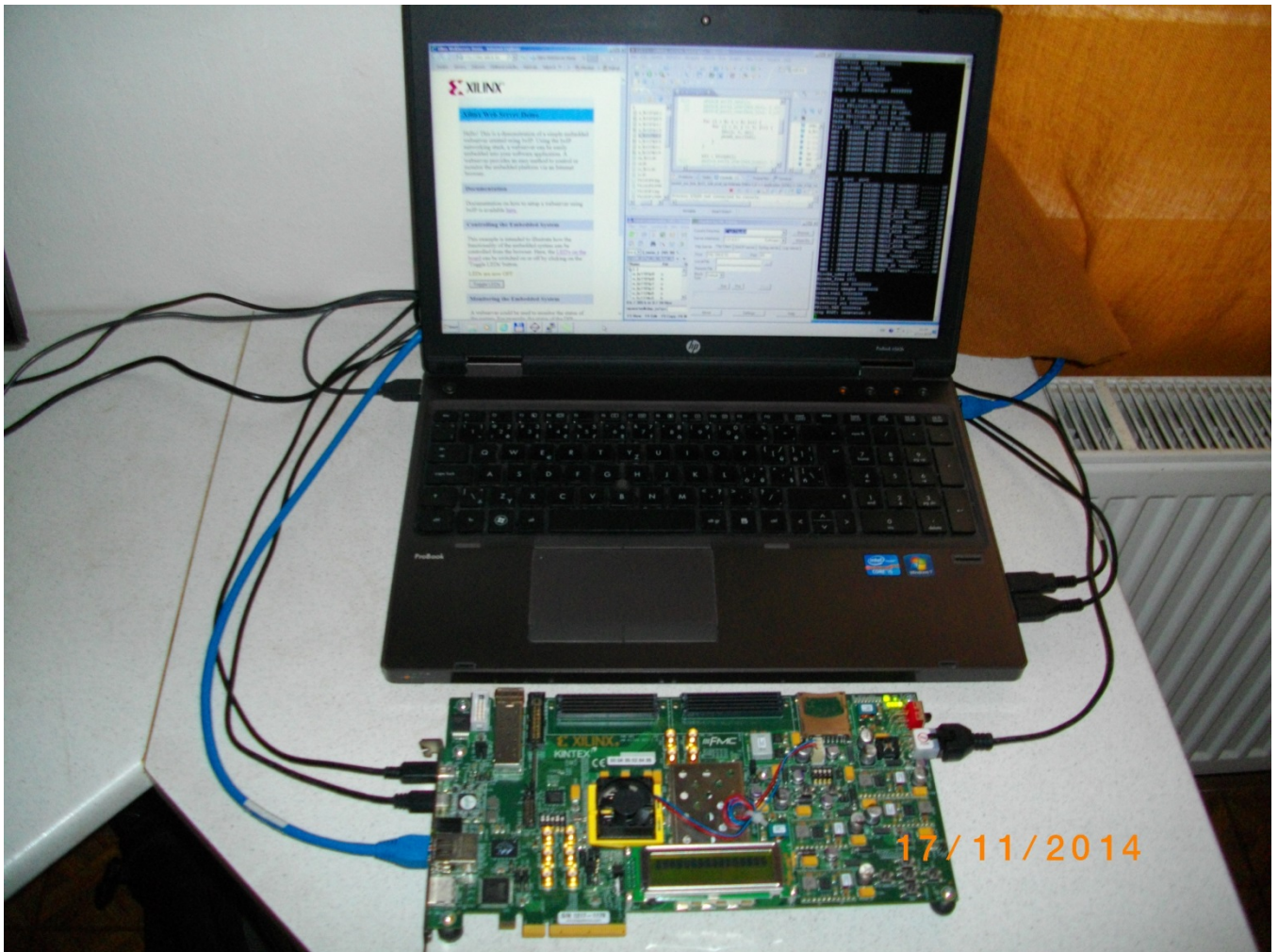
Photo 1: Demonstration of 1 Gb ethernet, www server and TFTP server with 8x (8xSIMD) EdkDSP floating point accelerators on Xilinx KC705 board with Kintex7 FPGA.
