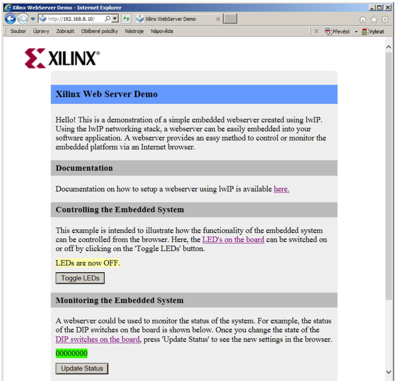
Figure 24: The demo www server is evaluating the basic GUI for communication from the web browser client to the Kintex7 application working as an embedded server providing 1 G bit point to point connection.
