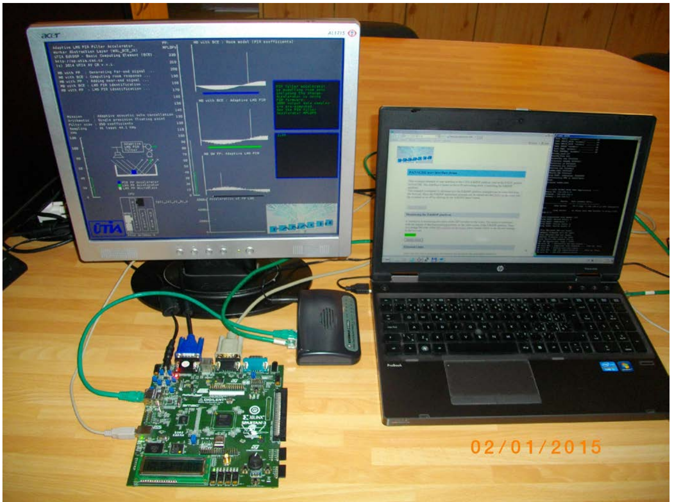
Figure 1: UTIA EdkDSP demonstrator with internet explorer GUI served from the 3S700AN kit
