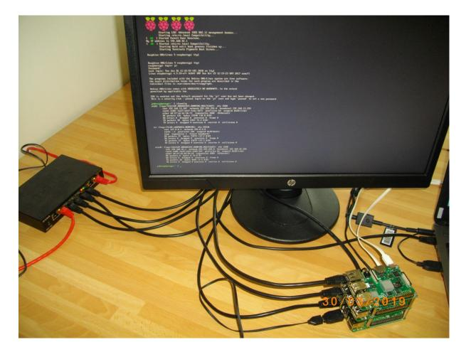
Figure 4: The RaspberryPi 3 will boot from the SD card, text output to monitor.
