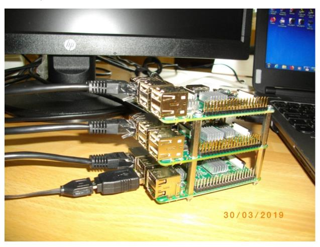
Figure 3: RPi3, Arrowhead G4.0 clients on two ZynqBerry boards
