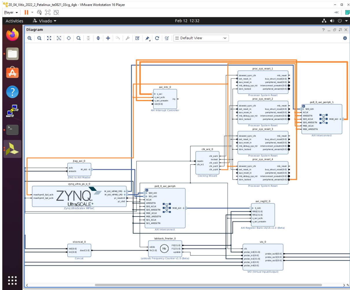
Double-click on **zynq\_ultra\_ps\_e\_0** to re-customize it by enabling of an interrupt input **pl\_ps\_irq0[0:0]**. Click OK.
