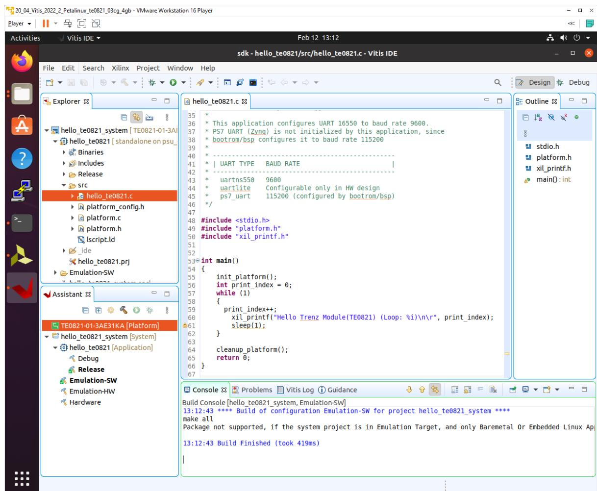
The TE0821-01-3AE31KA Vitis platform includes Trenz Electronic custom first stage boot loader in folder zynqmp\_fsbl. It includes SW extension specific for the Trenz module initialisation.
