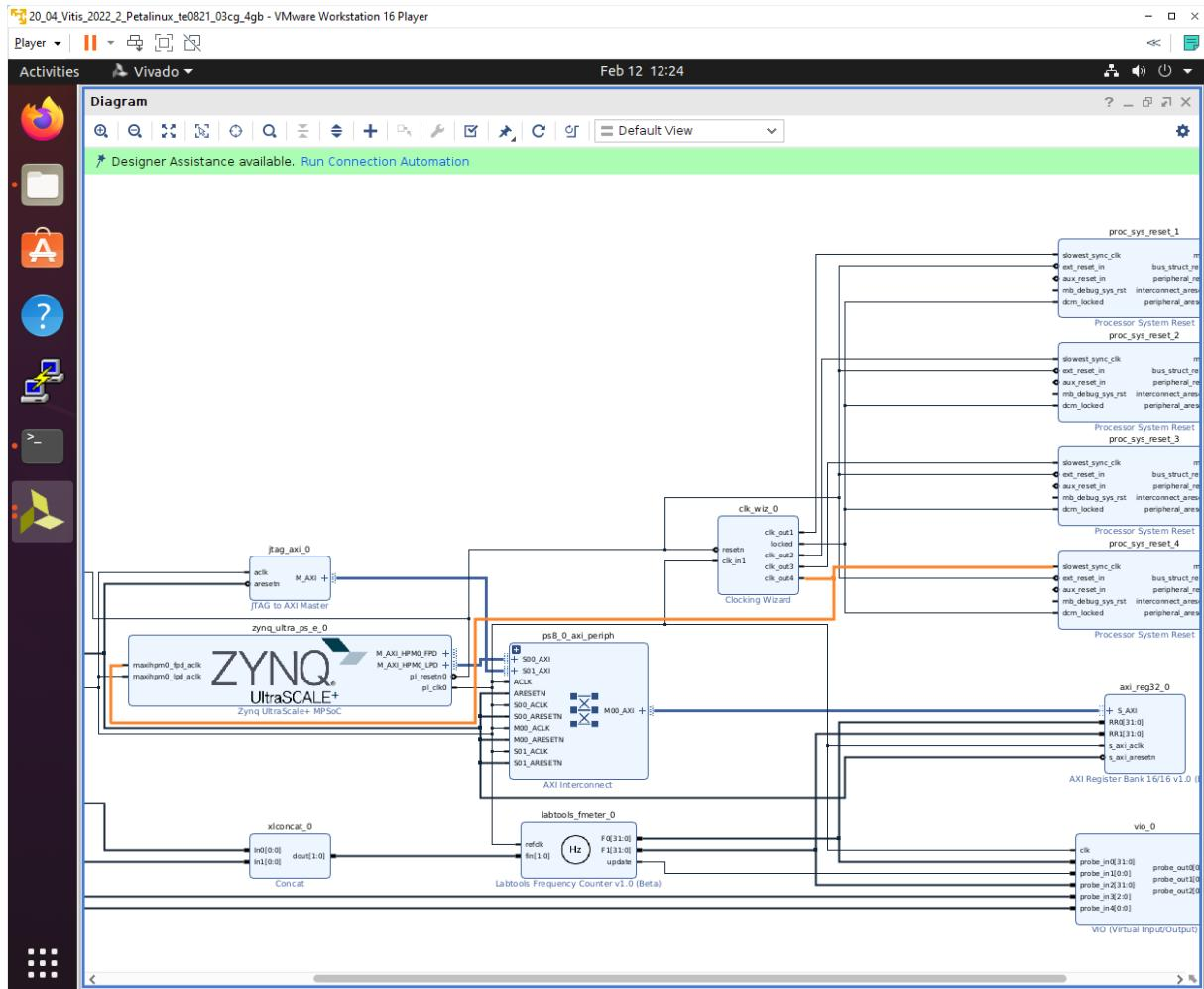
Double-click on **zynq\_ultra\_ps\_e\_0** block and enable **M\_AXI\_HPM0\_FPD** port. Select data width 32bit. It will be used for integration of interrupt controller on new dedicated AXI stream subsystem with 240 MHz clock. It will also enable new input pin **maxihpm0\_fpd\_aclk** of **zynq\_ultra\_ps\_e\_0**. Connect it to 240 MHz clock net.
