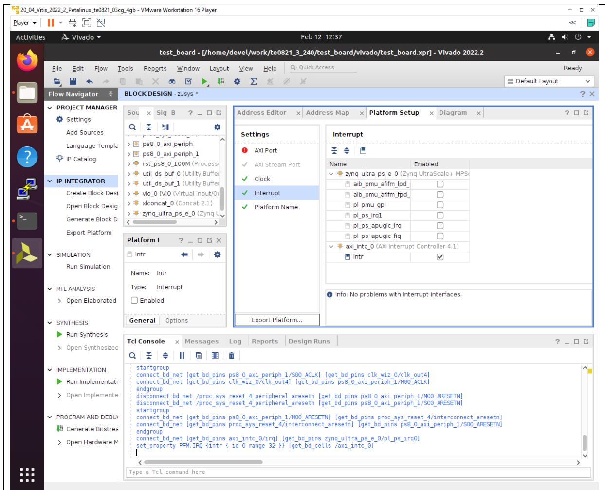
Rename automatically generated name **ps8\_0\_axi\_periph** of the interconnect to new name: **axi\_interconnect\_1**. This new name will be used in Platform Setup selection of AXI ports for the extensible platform.
