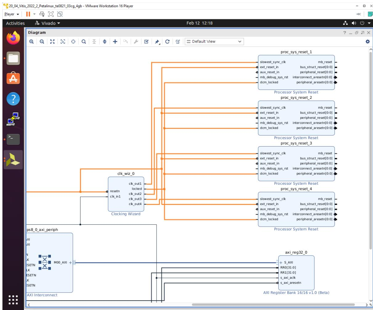
Open **Platform Setup** window of IP Integrator to define Clocks. In **Settings**, select **Clock**.
