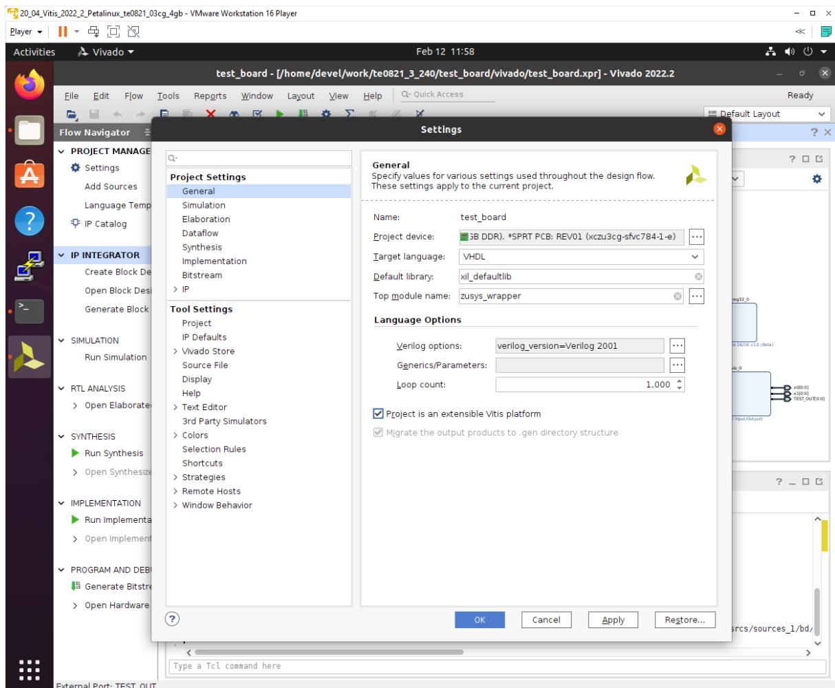
IP Integrator of project set up as an extensible Vitis platform has an additional Platform Setup window.
