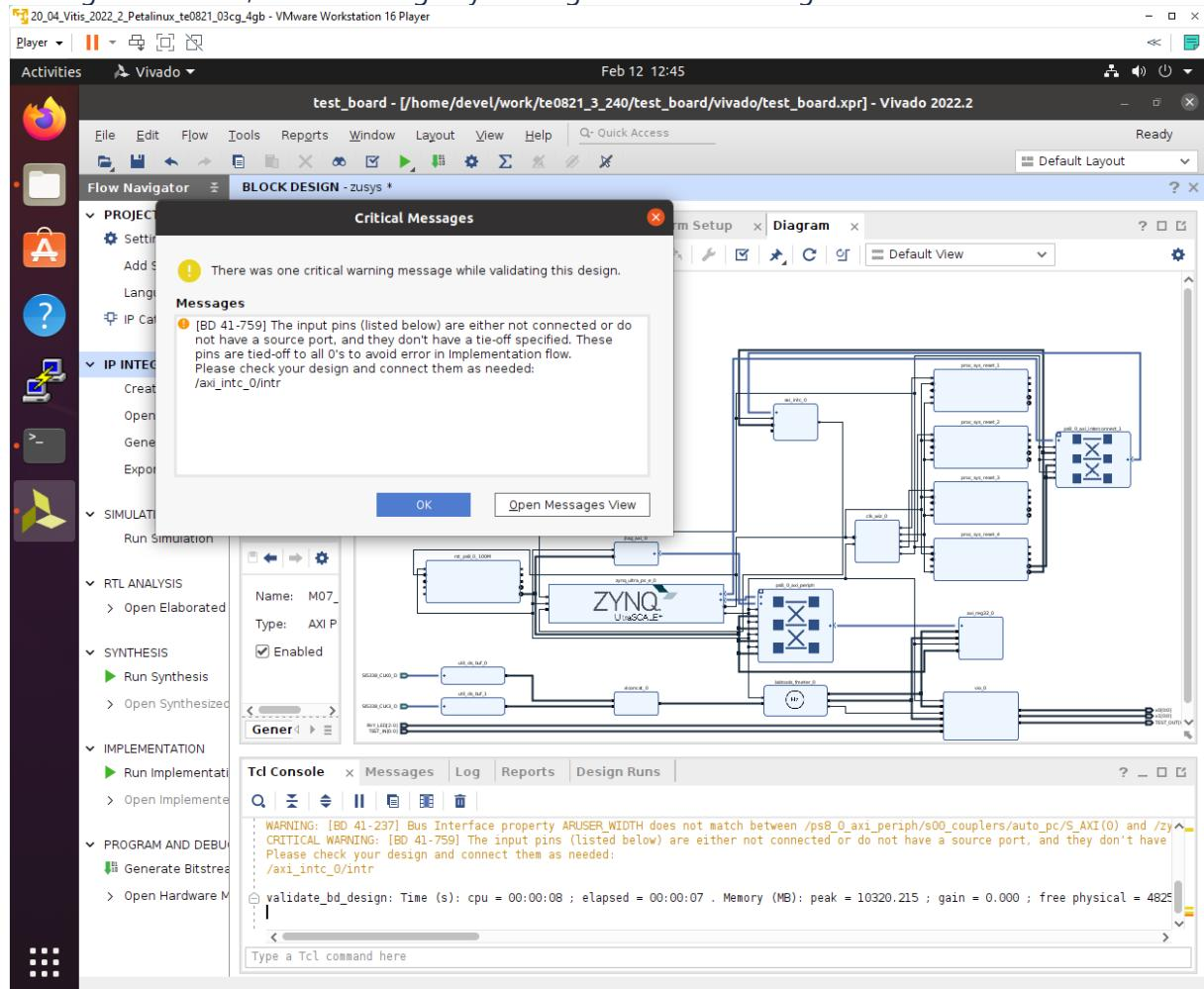
Received Critical Messages window indicates that input intr[0:0] of axi\_intc\_0 is not connected. This is expected. The Vitis extensible design flow will connect this input to interrupt outputs from generated HW IPs.
