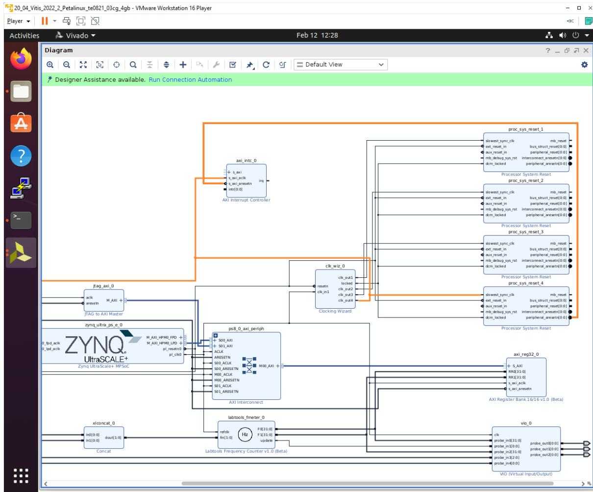
Use the **Run Connection Automation** wizard to connect the axi lite interface of interrupt controller **axi\_intc\_0** to master interface **M\_AXI\_HPM0\_FPD** of **zynq.ultra\_ps\_e\_0**.
