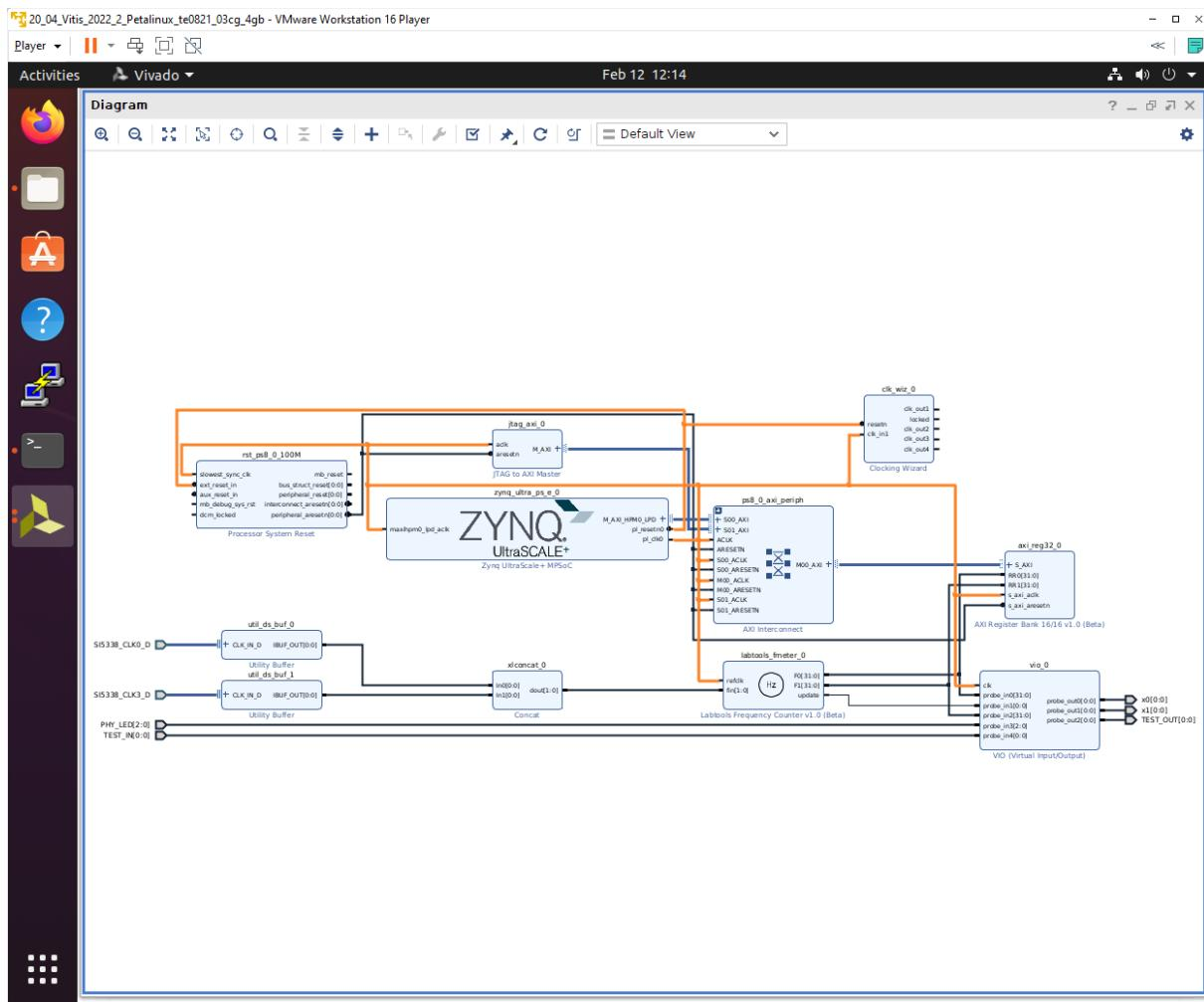
Add and connect four Processor System Reset blocks for each generated clock.
