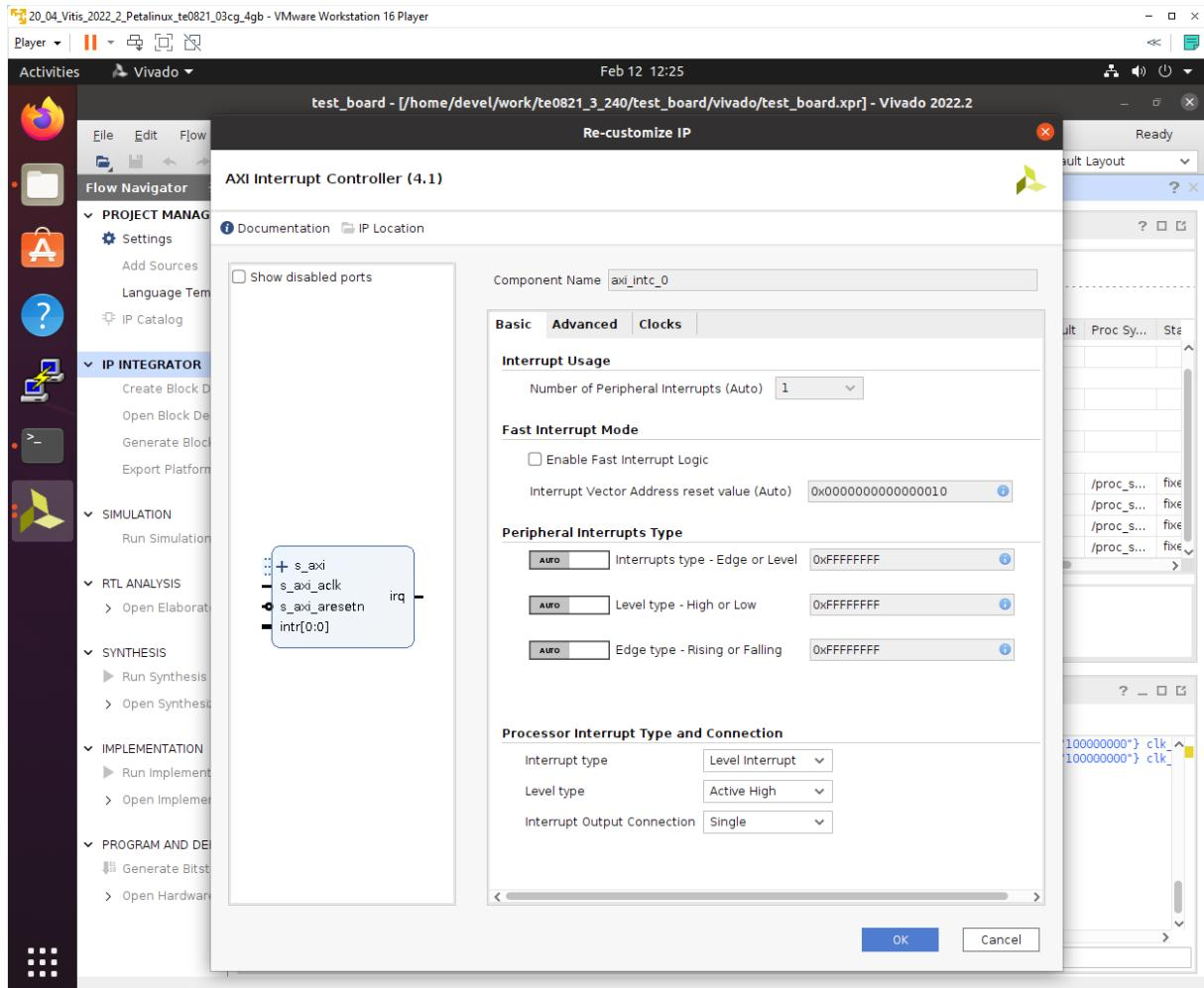
Connect interrupt controller clock input **s\_axi\_aclk** of **axi\_intc\_0** to output **dlk\_out4** of **clk\_wiz\_0**. It is the default, 240 MHz clock of the extensible platform.
