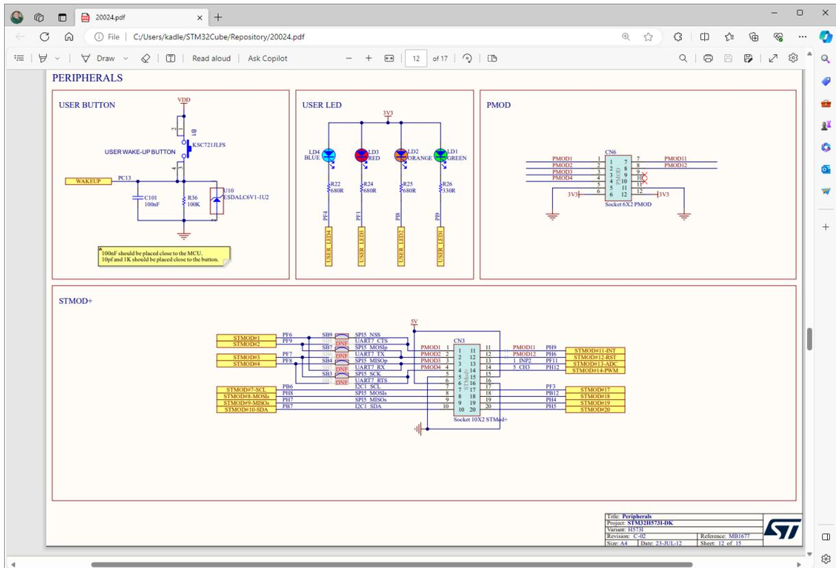
Reset wire connected to pin 7 of PMOD connector (PMOD11) is driven by pin PH9 of the STM32H5 device.
