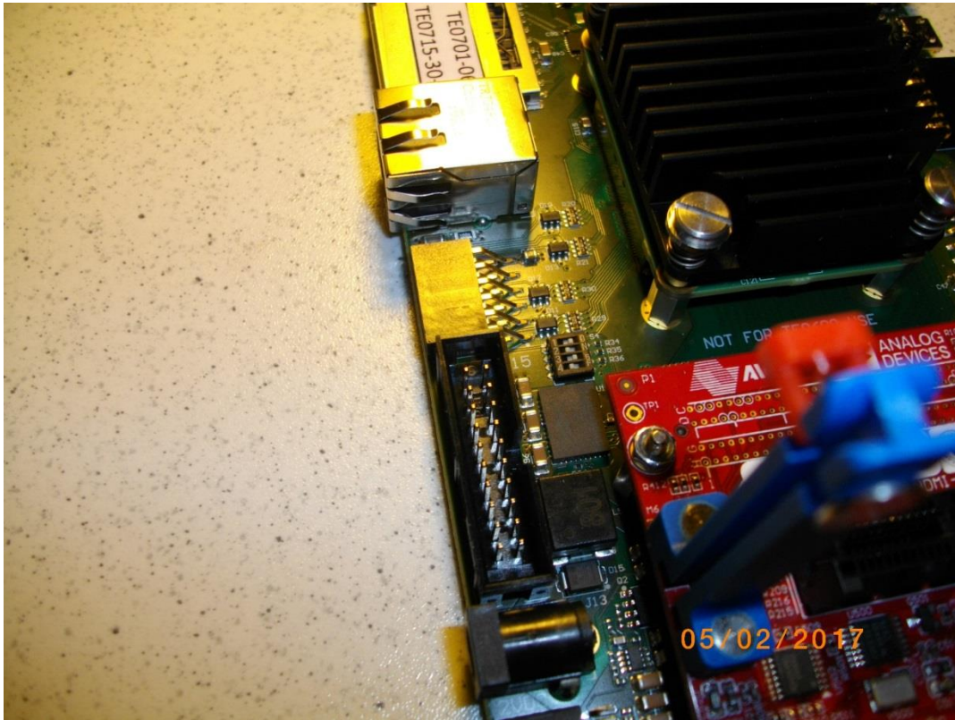
Figure 17: TE0701-06 setting of switch S4 (VADJ=1.8V): 1=ON 2=OFF 3=ON 4=OFF
