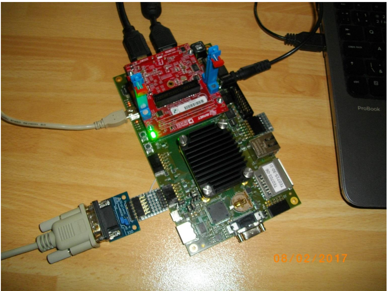
Figure 1: TE0701-06 carrier with TE0715-03-30-1 running HDMII-HDMI in HW and 3x EdkDSP accelerators.
