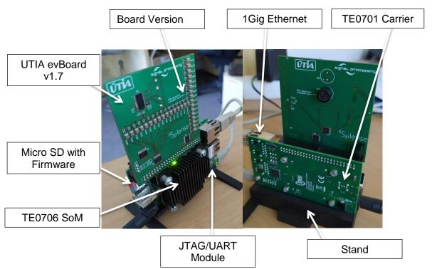
Figure 1: UTIA evBoard with FPGA module and carrier board.
