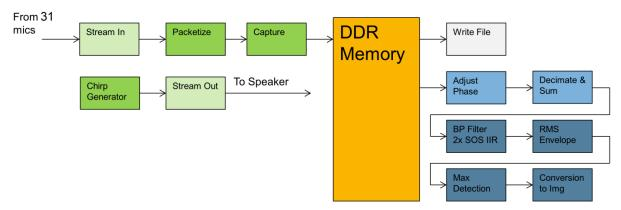
Figure 2: FPGA implementation of the beamformer accelerators
